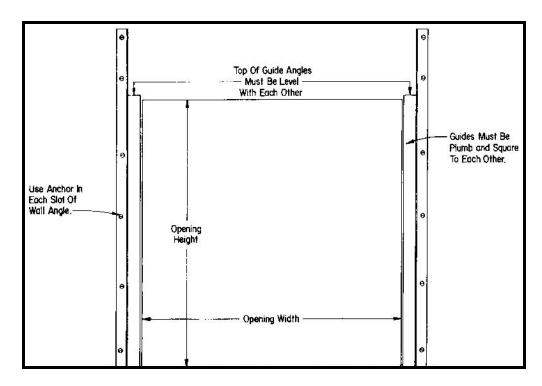
STEP 8 LOCATING GUIDE ASSEMBLIES. Locate guide assemblies such that "R" Dimension exists between guides as shown. Bottom of guides MUST be on a level line and Guides MUST be plumb.
