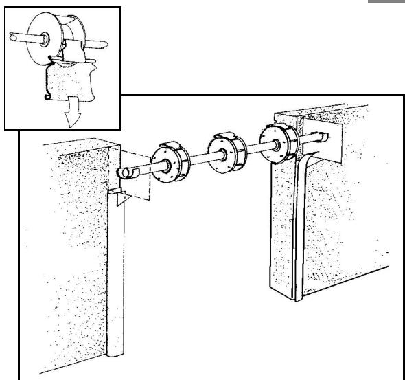
TAKE EXTREME CAUTION WITH PIN ATTACH TO SPRING BOX. DO NOT RE-MOVE PIN UNTILL CURTAIN IS ENGAGE TO SPRING BOX.
